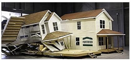
Engineers at the Insurance Institute for Business & Home Safety research center can blast homes with tornado-strength winds generated by 105 giant fans. Drop in a half-million gallons of water or ice from the ceiling, and they can simulate hurricanes and hailstorms.
